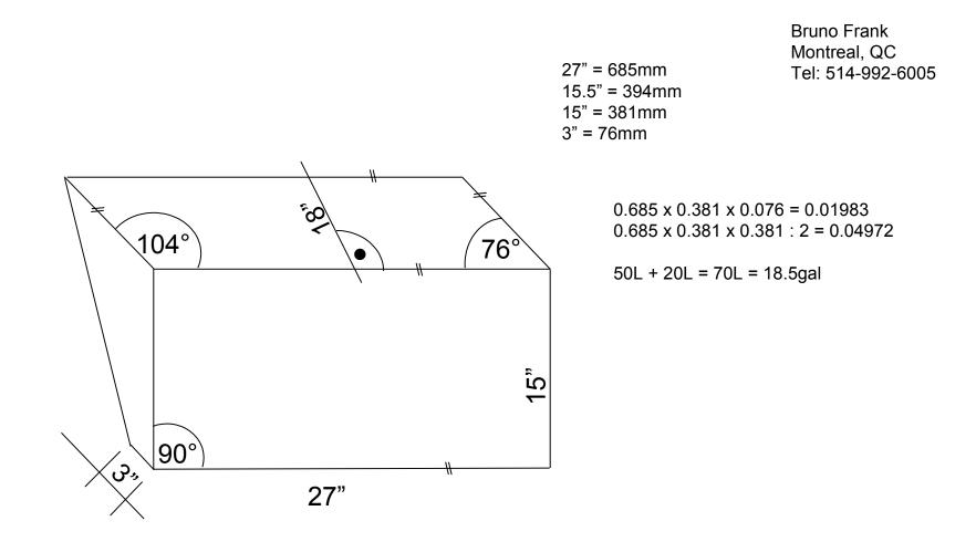
On the outside measure, this tank has a total of 18.5gal. Inside, with a wall thickness of 3/8, I estimate about 17.5gal. Maximum capacity (not calculated).
