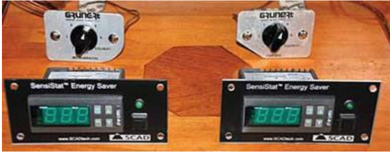
Similar products tested by Practical Sailor include the manual Frigoboat Speed Board controller (top photo; $38; June 2009), and the programmable automatic Sensistat (bottom photo; $300; April 2009), which was tested with a holding-plate fridge system.
